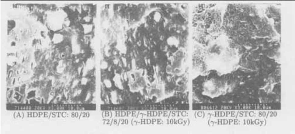
Fig. 9 SEM of liquid nitrogen frozen fractured surface of specimens
